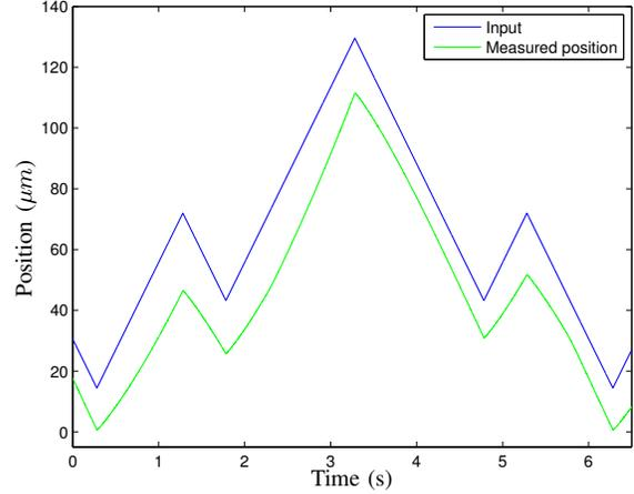
Fig. 2. Experiment where a triangular wave with varying amplitude is applied as input to the piezo actuator. The hysteretic behavior is clearly visible in the response.
