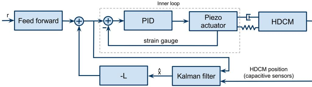
Fig. 8. Control structure for model-based control of the HDCM, where each Cartesian axis is considered separately.
