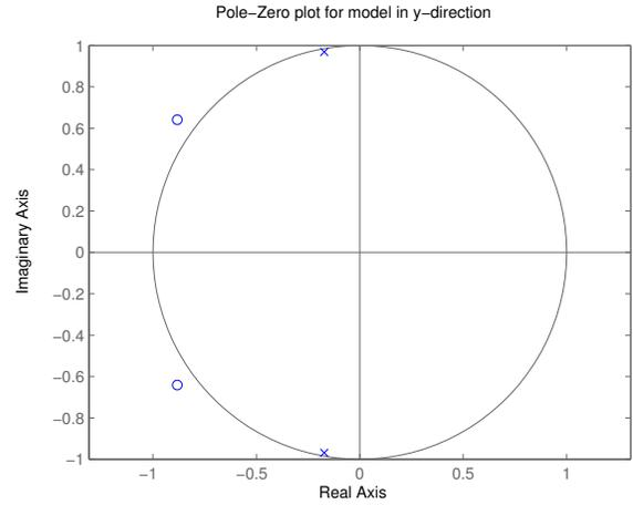
Fig. 7. Pole-zero plot for the identified state-space model in the  $y$ -direction.
