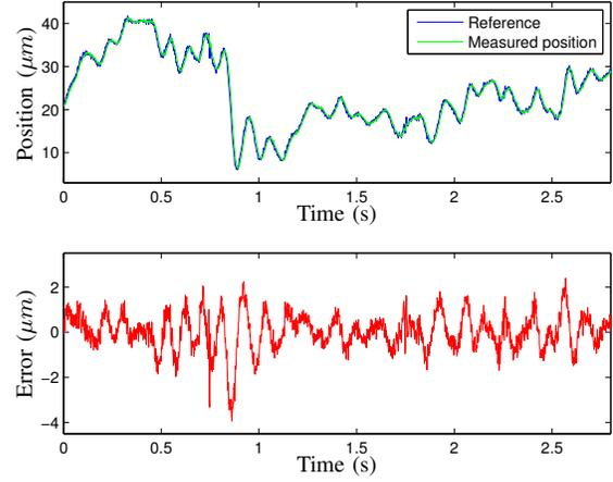
Fig. 11. Control performance in the inner PID control loop in the  $y$ -direction.
