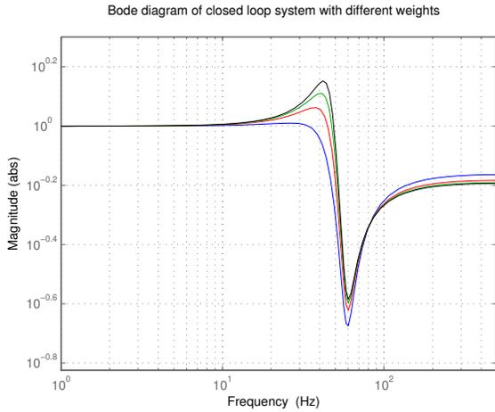
Fig. 10. Bode diagram for the closed loop system for  $Q = I$  and different choices of the  $R$ -matrix in the LQ-design. The choices of  $R$  are 1.0, 2.0, 3.0 and 4.0 for the blue, red, green and black line, respectively.
