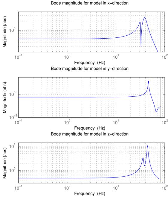
Fig. 5. Bode magnitude of the discrete-time state-space models identified using sub-space identification, in the  $x$ -  $y$ - and  $z$ -directions, respectively.
