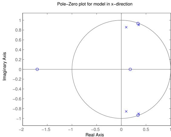
Fig. 6. Pole-zero plot for the identified state-space model in the  $x$ -direction.
