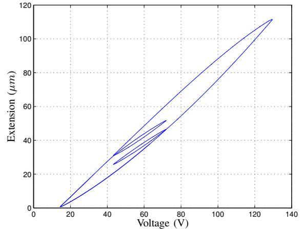
Fig. 3. Extension of the piezo actuator as function of the input for the experiment in Fig. 2. Note the complex behavior of the hysteresis, which exhibits both rate and amplitude dependency.
