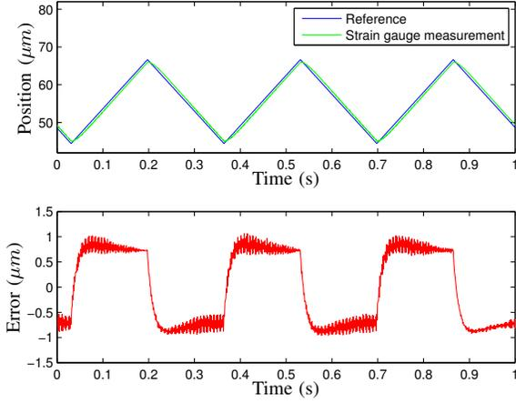
Fig. 9. Performance of the inner PID control loop in the  $y$ -direction when applying a 3 Hz triangular wave as input.
