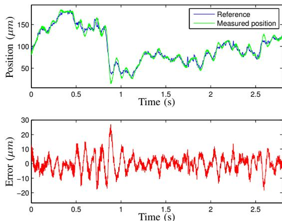
Fig. 12. Performance of the model-based spindle positioning control in the  $y$ -direction.
