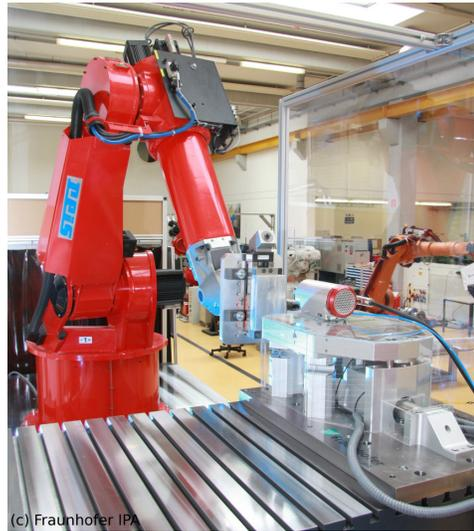
Fig. 1. The experimental setup for real-time compensation of positioning errors during machining operations, where the robot holds the workpiece and the spindle holding the milling tool is mounted on the HDCM-unit.
