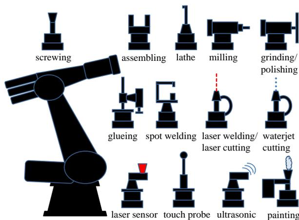
Figure 7 – Smart Robot Tooling Concept
