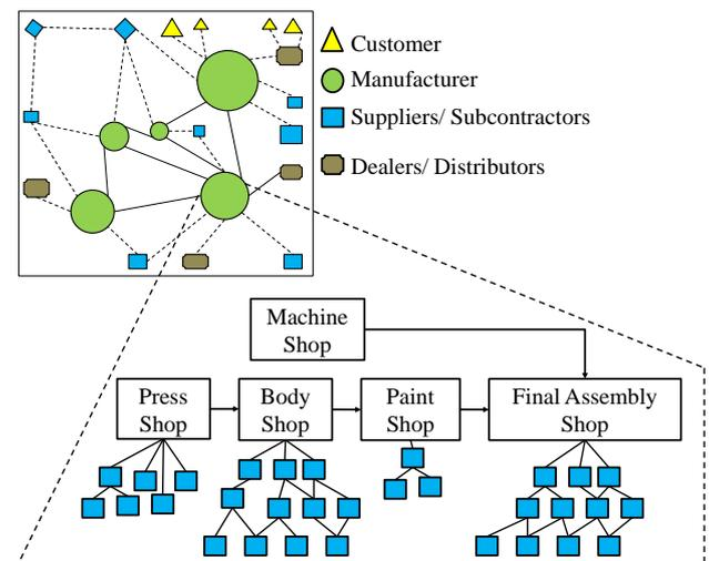
Figure 2 – Distributed Manufacturing System (Network and Automobile Manufacturing Phases)
