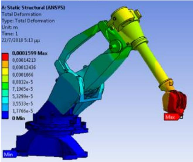
Figure 3b : Contours of Total Deformation (applied force of 500N, supported at base)
