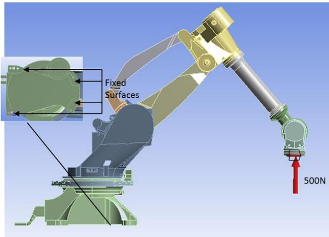
Figure 2: Force application vector and applied constraints
