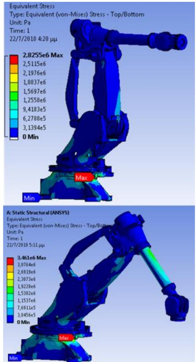
Figure 3a : Contours of Equivalent Stress (applied force of 500N, supported at base)
