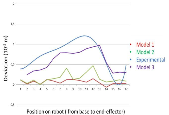
Figure 4: Comparison of experimental data to FE results
