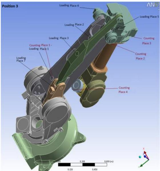
Figure 5 : Model in position No.3 – Load and measuring points are displayed
