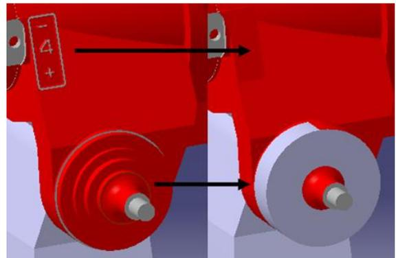
Figure 1 : Illustration of simplifications (right) performed on the robot model
